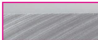
SUMICRYSTAL (Single-crystal Diamond) SC10 Wiper Blade Machined Surface
