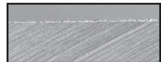
SUMIDIA (Sintered Diamond) Wiper Blade Machined Surface
